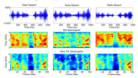
Fig. 2. (Color online) Comparison of the spectrographic representation provided by mel frequency analysis and the proposed modulation filtering approach for a clean speech signal, noisy speech signal (additive babble noise at 10 dB SNR) and radio channel speech (non-linear noise from channel C).
