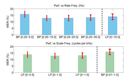
Fig. 3. (Color online) ASR performance in terms of word error rate [WER (%)] with standard deviation (error bar) as a function of the rate frequency (Hz) and scale frequency (cycles per kHz). Here, LP denotes low-pass filtering, BP denotes band-pass filtering, and the two frequencies in the x axis indicate the lower and upper cut-off frequency.
