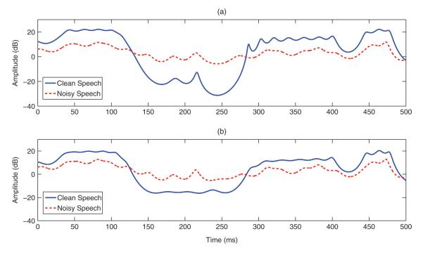
FIG. 3. (Color online) Log-FDLP envelopes for a sub-band of clean speech and speech corrupted with babble noise at 10 dB SNR. (a) Without noise compensation and (b) with noise compensation.
