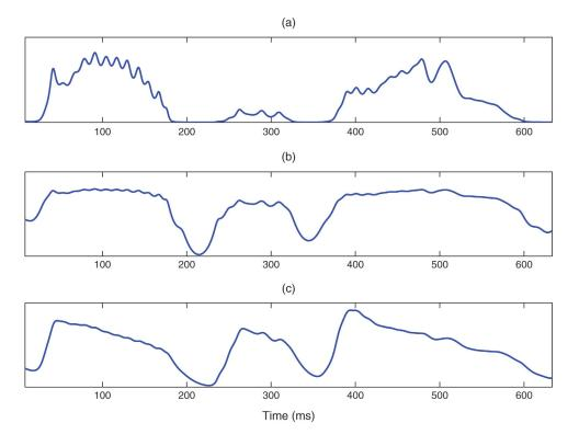
FIG. 8. (Color online) Static and dynamic compression of the FDLP envelopes. (a) A portion of sub-band FDLP envelope, (b) logarithmic compression of the FDLP envelope, and (c) adaptive compression of the FDLP envelope.
