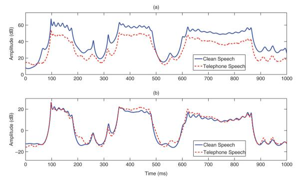
FIG. 5. (Color online) Log-FDLP envelopes for a sub-band of clean speech and telephone speech. (a) Without gain normalization and noise compensation, and (b) with gain normalization and noise compensation.
