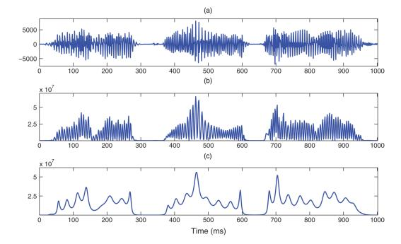
FIG. 2. (Color online) Illustration of the all-pole modeling property of FDLP. (a) A portion of the sub-band speech signal (with frequency range of 500– 700 Hz), (b) its Hilbert envelope, and (c) all-pole model obtained using FDLP with model order of 80.
