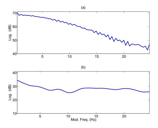
Figure 3.1: (a) Spectrum of a clean speech envelope for a narrow-band signal (b) Spectrum of a typical room-response envelope for a narrow-band signal (small dynamic range).
