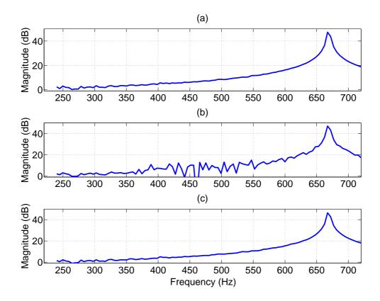
Figure 6.5: Improvements in reconstruction signal quality with SNS: A portion of power spectrum of (a) a tonal input signal, (b) reconstructed signal using the base-line FDLP codec without SNS, and (c) reconstructed signal using the FDLP codec with SNS.
