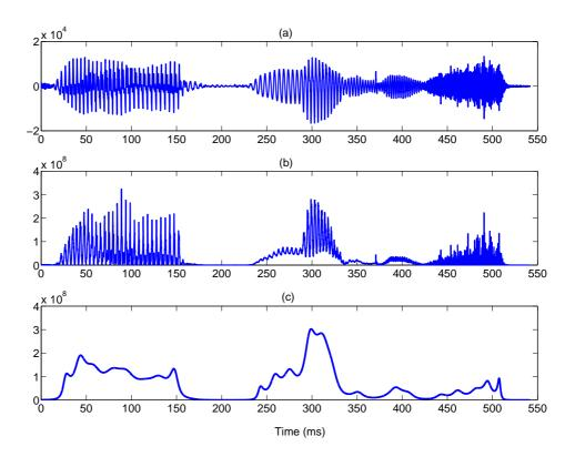
Figure 2.4: Illustration of the AR modeling property of FDLP. (a) a portion of speech signal, (b) its Hilbert envelope and (c) all pole model obtained using FDLP.
