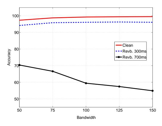
Figure 4.9: Word recognition accuracy as function of the bandwidth of the sub-band for clean and two types of reverberant data.
