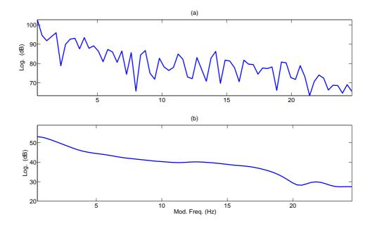
Figure 3.2: (a) Spectrum of a clean speech envelope for a wide-band decomposition (b) Spectrum of a typical room-response envelope for a wide-band decomposition (large dynamic range compared to Fig. 3.1 (b)).
