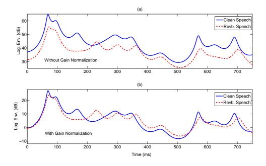
Figure 3.4: Log FDLP envelopes for clean and reverberant speech for sub-band 750 - 850 Hz. (a) without gain normalization (b) with gain normalization.
