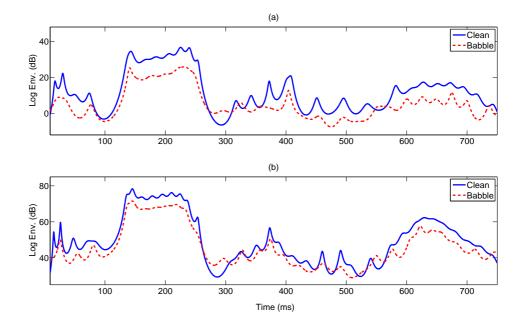
Figure 2.8: Log FDLP envelopes from clean and noisy (babble at 10 dB) sub-band speech. (a) Low resolution envelopes and (b) High resolution envelopes.
