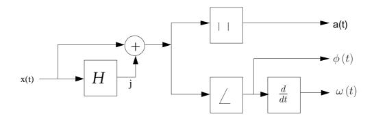
Figure 2.1: Demodulation procedure using analytic signal.
