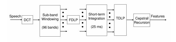
Figure 7.1: Block schematic of 2-D AR model based feature extraction.
