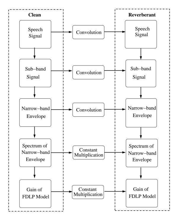
Figure 3.3: Summary of the assumptions made for reverberant signal. The effect appears as a modification of the gain of the sub-band FDLP model in narrow bands.
