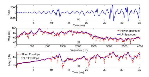
Figure 2.3: (a) A portion of speech signal, (b) Spectral AR model (TDLP) and (c) Temporal AR model (FDLP).
