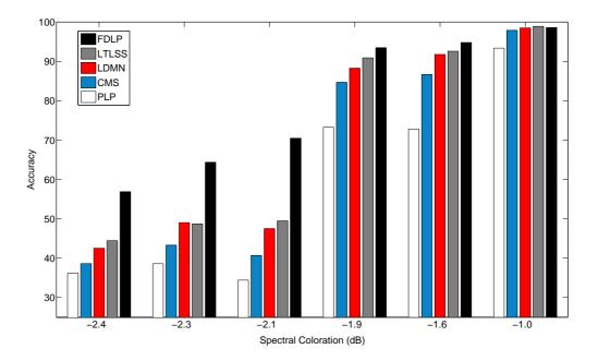
Figure 4.12: Comparison of word recognition accuracies (%) using different techniques using 6 artificial room responses.
