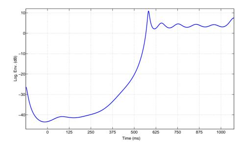
Figure 4.4: FDLP envelope of the sub-band around 2 kHz for the signal in Fig. 4.2 with a FDLP model order of 20 poles per second.
