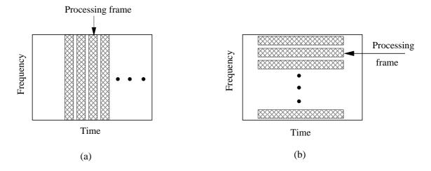
Figure 1.1: Overview of time-frequency energy representation for (a) conventional analysis and (b) proposed analysis.
