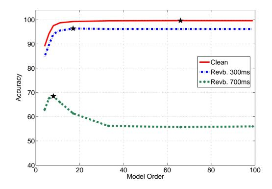
Figure 4.10: Word recognition accuracy as function of the model order for clean and two types of reverberant data. The best performance in each condition is highlighted using the star sign.
