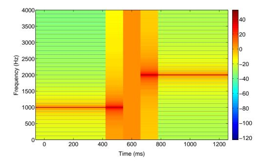
Figure C.2: Narrow-band STFT spectrogram for the signal in Fig. 4.2 using 200 ms window with half overlap.
