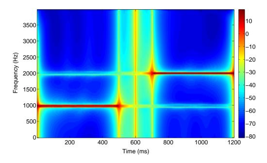
Figure 4.3: FDLP spectrogram for the signal in Fig. 4.2 using 120 sub-bands and FDLP model order of 20 poles per sub-band per second.
