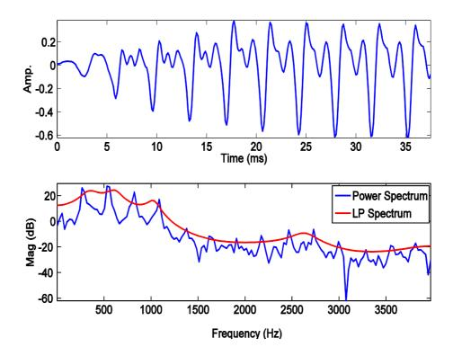
Figure 2.2: Illustration of the all-pole modeling property of the TDLP model. (a) Portion of speech signal, (b) Power spectrum and the TDLP approximation.
