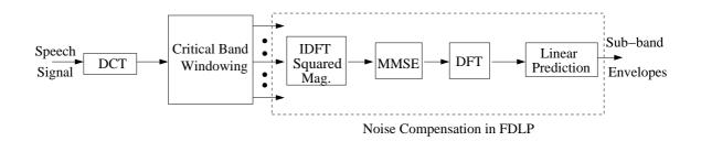
Figure 5.4: Block schematic for noise compensation in FDLP.
