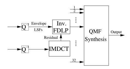
Figure 6.2: Scheme of the FDLP Decoder.
