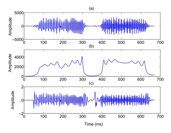
Figure 2.5: Illustration of AM-FM decomposition using FDLP. (a) a portion of band pass filtered speech signal, (b) its AM envelope estimated as square root of FDLP envelope and (c) the FDLP residual containing the FM component.
