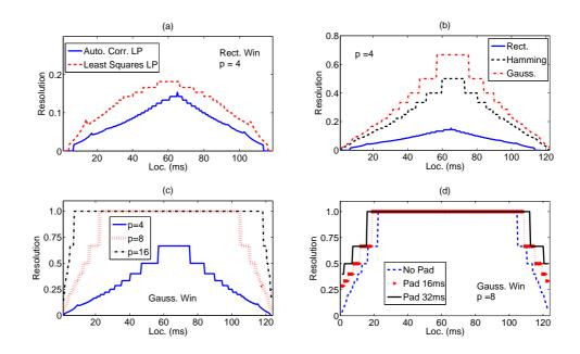
Figure 2.7: Normalized resolution in FDLP as function of the location of the first peak for a 125 ms long signal. (a) Two LP methods, (b) Various DCT windows, (c) FDLP model order and (d) symmetric padding at the boundaries.
