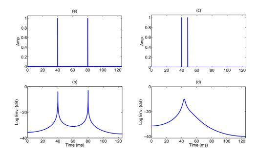
Figure 2.6: Plot of 125 ms of input signal in time domain (a), (c) and the corresponding log FDLP envelopes (b), (d).
