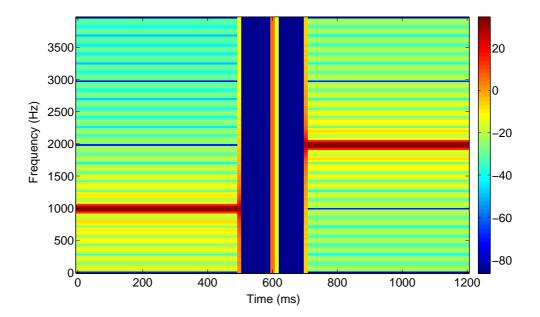
Figure C.1: Wide-band STFT spectrogram for the signal in Fig. 4.2 using 25 ms window with half overlap.
