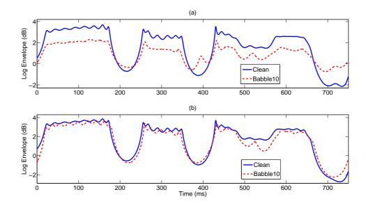
Figure 5.5: Gain normalized sub-band FDLP envelopes for clean and noisy speech signal (babble 10 dB) (a) without and (b) with MMSE noise suppression.
