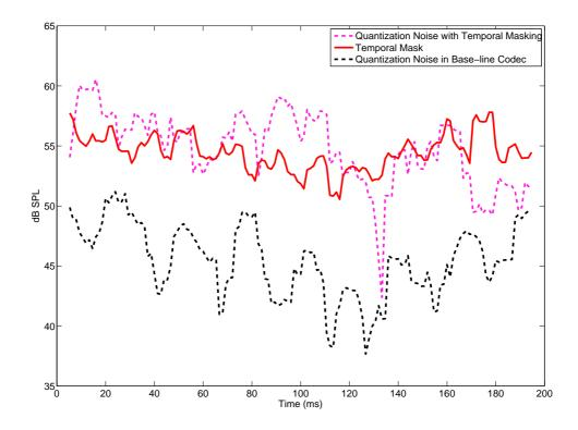
Figure 6.3: Application of temporal masking to reduce the bits for 200ms region of a subband signal. The figure shows the temporal masking threshold, quantization noise for the codec without and with temporal masking.
