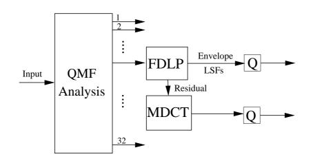
Figure 6.1: Scheme of the FDLP encoder.
