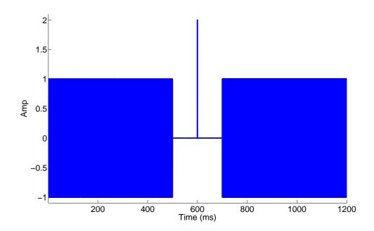
Figure 4.2: An experimental signal with impulsive nature in time-frequency domain used for the resolution analysis of FDLP spectrogram.
