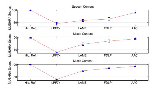
Figure 6.6: MUSHRA results for each audio sample type namely speech, mixed and music content obtained using three coded versions at 48 kbps (FDLP-MDCT (FDLP), MPEG-4 HE-AAC (AAC) and LAME-MP3 (LAME)), hidden reference (Hid. Ref.) and 7 kHz low-pass filtered anchor (LPF7k) with 8 listeners.
