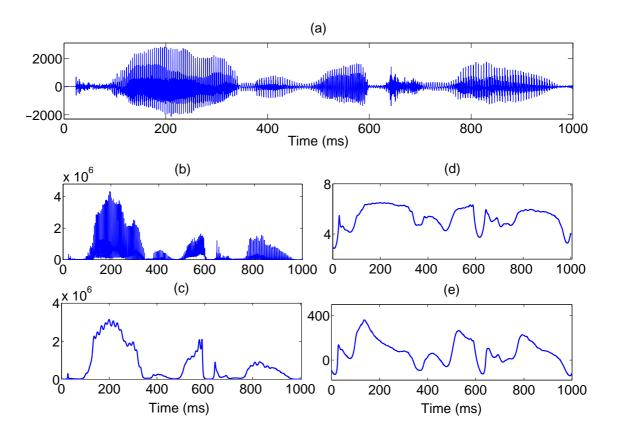
Figure 5.3: Static and dynamic compression of the temporal envelopes: (a) a portion of 1000 ms of full-band speech signal, (b) the temporal envelope extracted using the Hilbert transform, (c) the FDLP envelope, which is an all-pole approximation to (b) estimated using FDLP, (d) logarithmic compression of the FDLP envelope and (e) adaptive compression of the FDLP envelope.
