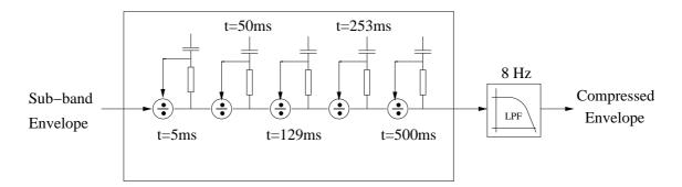
Figure 5.2: Dynamic compression of the sub-band FDLP envelopes using adaptive compression loops.
