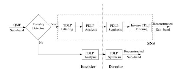
Figure 6.4: Sub-band processing in FDLP codec with SNS.
